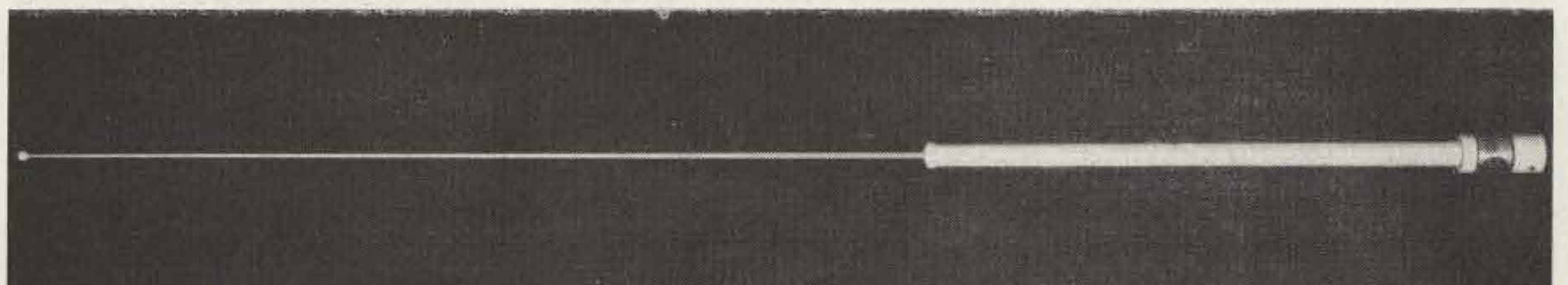
Fig. 10. Sleeve-decoupled half-wave whip designed for marine VHF use.
